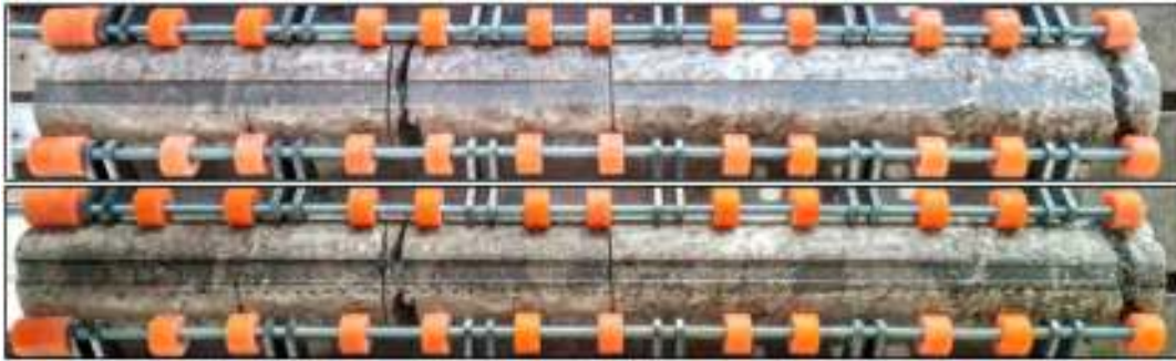
Figure 1—The full-size core at different test stages: top - after grinding, bottom - after a measuring cutter run
